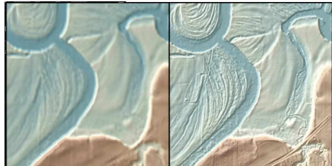
Left: Shaded relief for a USGS 10-meter DEM. Right: 2007 airborne LiDAR imagery, Pecatonica River, Winnebago County, with higher spatial and vertical resolution.
