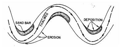
Figure 1- 4: Erosion changes the shape of channels
