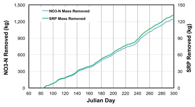
Based on the measured flowrates and inlet/outlet nutrient concetrations, the cumulative N and P removal was determined using a mass balance approach.
