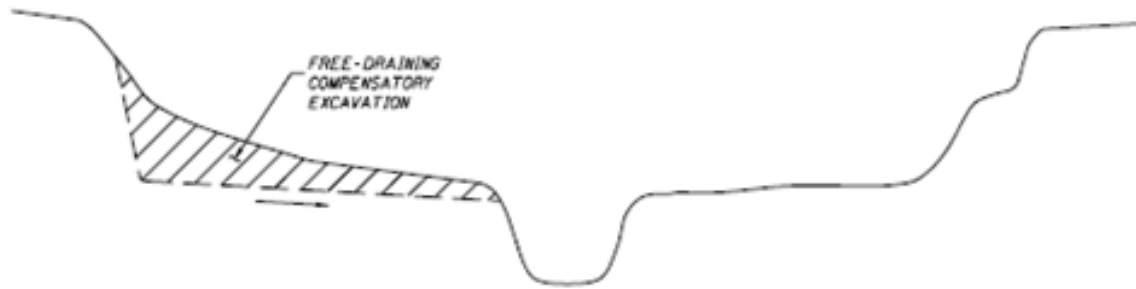
Figure 4.3(a): Cross-section of free draining compensatory excavation
