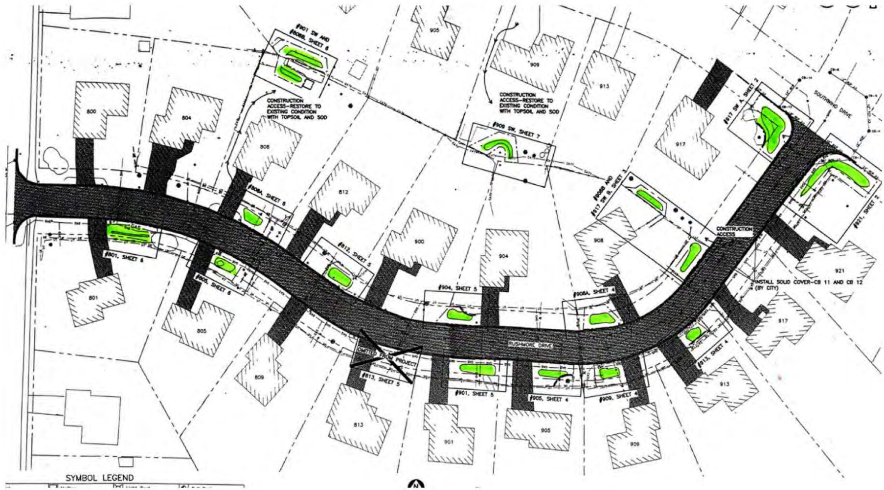
Figure 2 Treatment Watershed Rainwater Garden Layout
