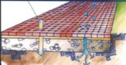
Permeable Pavers, Green Alley Handbook, Chicago Department of Transportation
