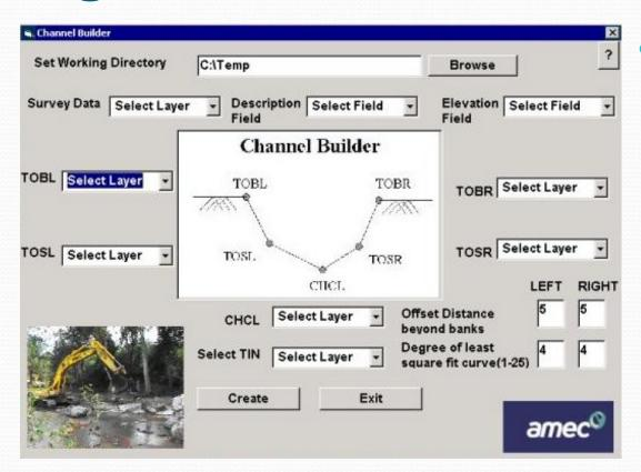
The Digital Channel Builder uses field survey data to 'burn' a channel into a digital ground surface. Makes hydraulic model creation easier and floodplain delineation smoother.
