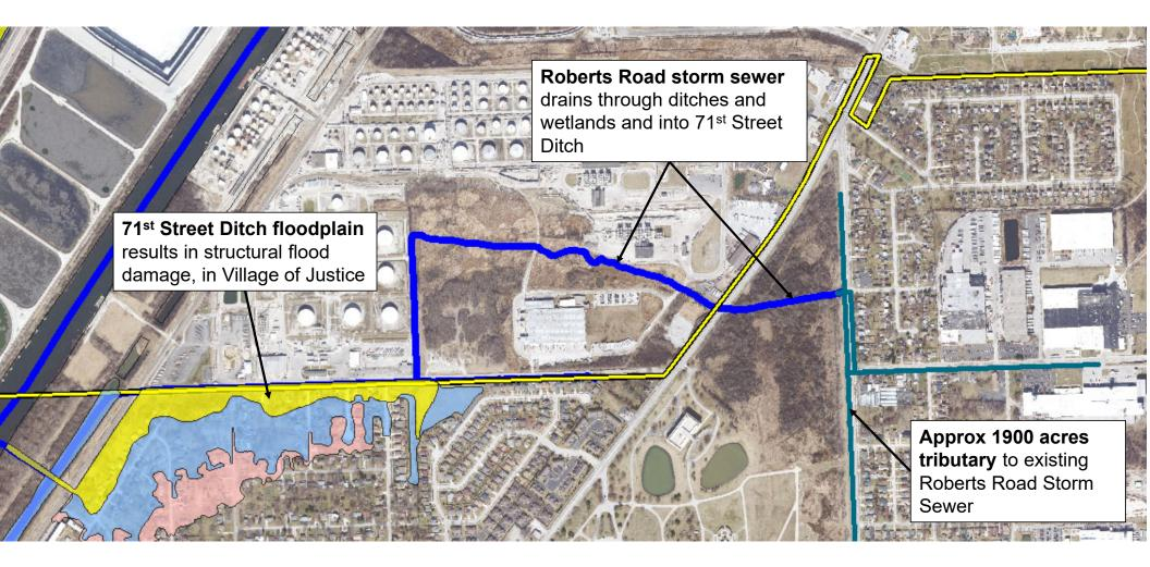
Limitations on New Discharges to 71st St Ditch: Proposed Conditions
