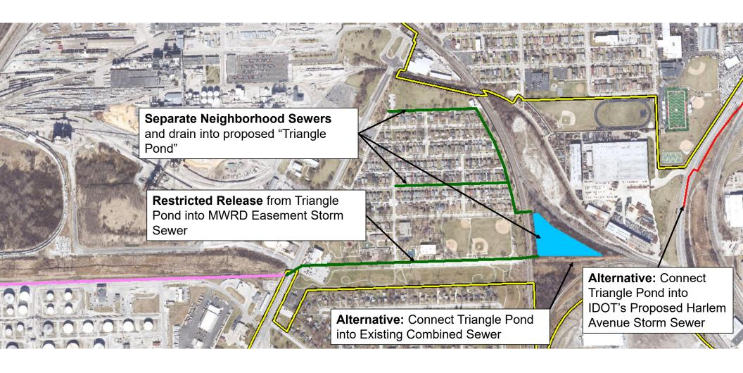
Limitations on New Discharges to 71st St Ditch: Existing Conditions
