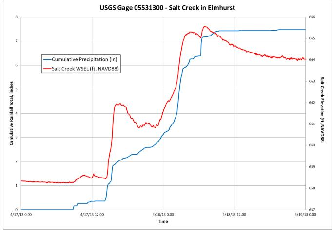
•As shown to the left for the April 2013 event, the level of Salt Creek rises rapidly during extreme storm events, which reduces the capacity of the existing storm sewer system.
