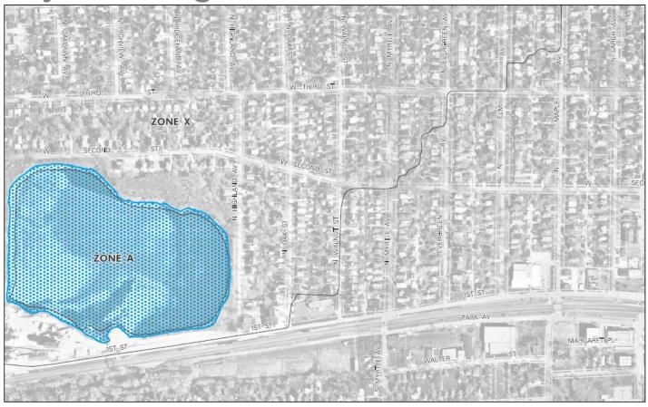
Although this area is not mapped as floodplain according to the Federal Emergency Management Agency (FEMA) Flood Insurance Rate Map (FIRM), it does show the location of a historic drainageway through the area. Today, the 60- to 72-inch diameter storm sewer is located in its place.
