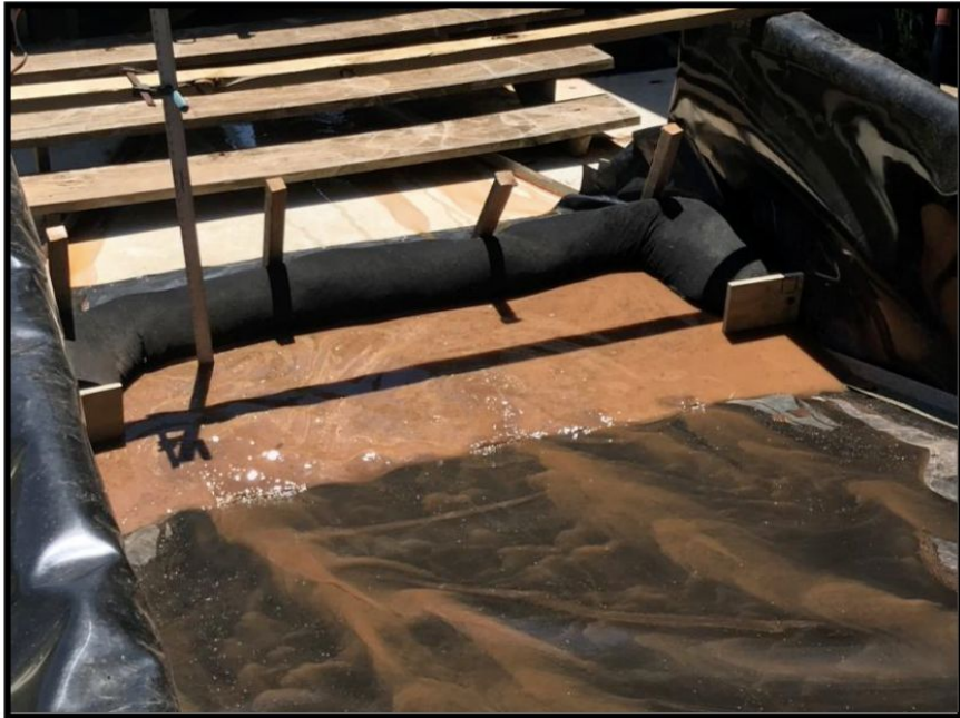
Ponding and Sediment Build-up Behind Wattle at end of Flow
