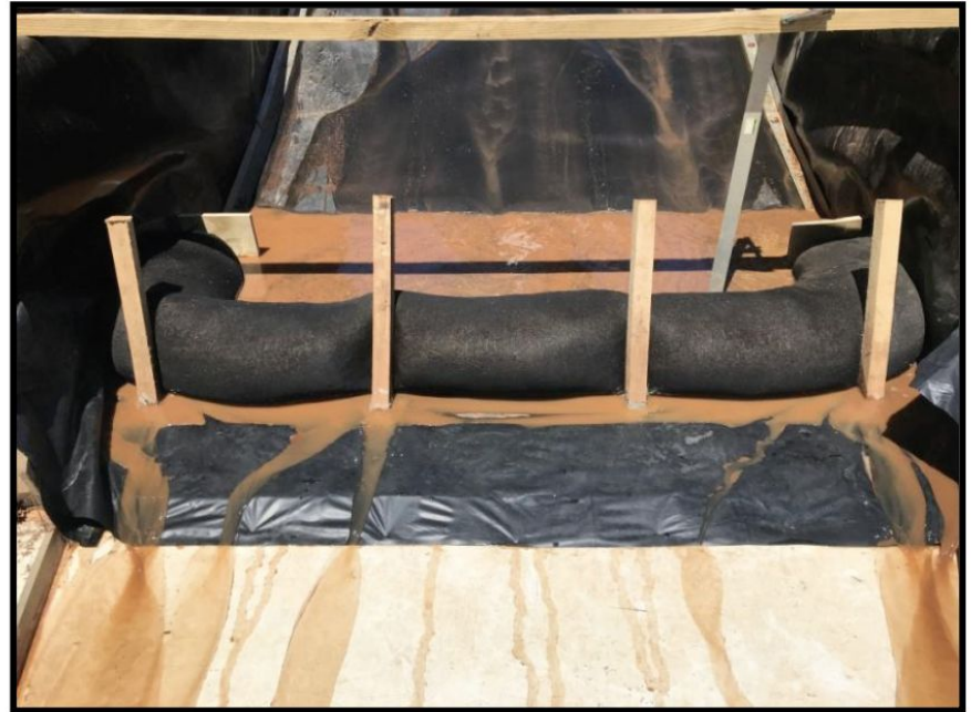
Ponding and Sediment Build-up Behind Wattle at end of Flow
